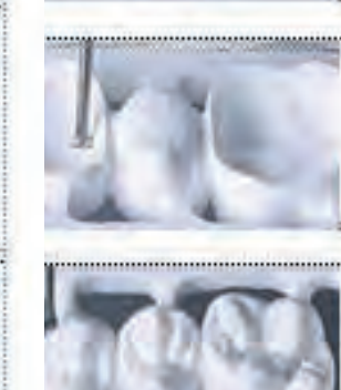
Milling Bur 1,5 A Used to mill pre-sintered zirconia (abutment)
